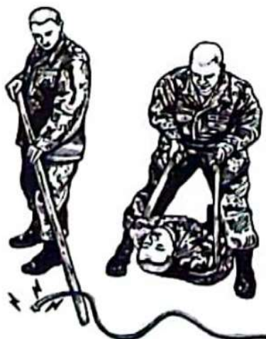
Figure 3-14. Casualty removed from electrical source (using nonconductive material).
